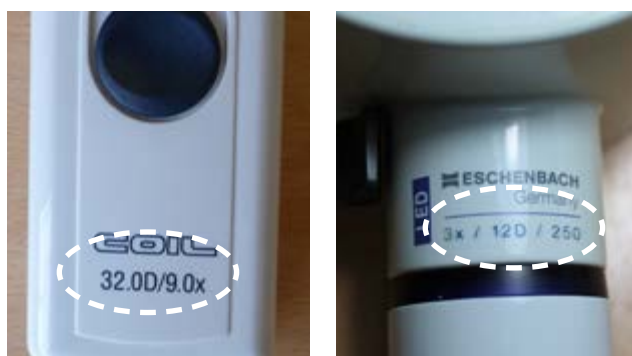
Figure 5.9 The device on the left side is labelled using trade magnification ( 32D/4 + 1 = 8 + 1 = 9x ), while the one on the right uses nominal magnification ( 12D/4 = 3x ).
