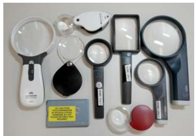
Figure 6.2 Hand magnifiers. They come in different shapes and powers, from 4D or 1x, up to 56D or 14x.
