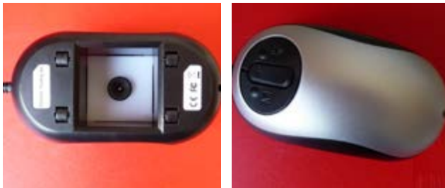
Figure 6.14 Mouse Magnifiers that can be connected to a home TV to create a basic electronic magnifier system.
