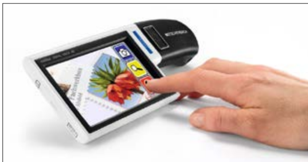
Figure 6.15 Hand held CCTV allows flexible control of magnification and contrast but these devices are expensive costing 10 – 20x the cost of a simple hand magnifier. Photo Associated Optical.
