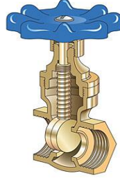
Figure (5): Gate Valve
