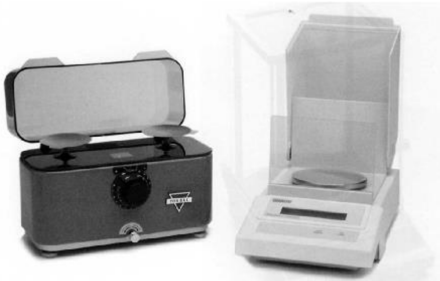
FIGURE 3.3 Torbal torsion balance and Chaus electronic balance. (Courtesy of Total Pharmacy Supply, Inc.)
