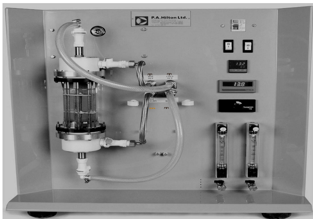
Fig. 5.1: Shell and tube heat exchanger connected to the service unit.
