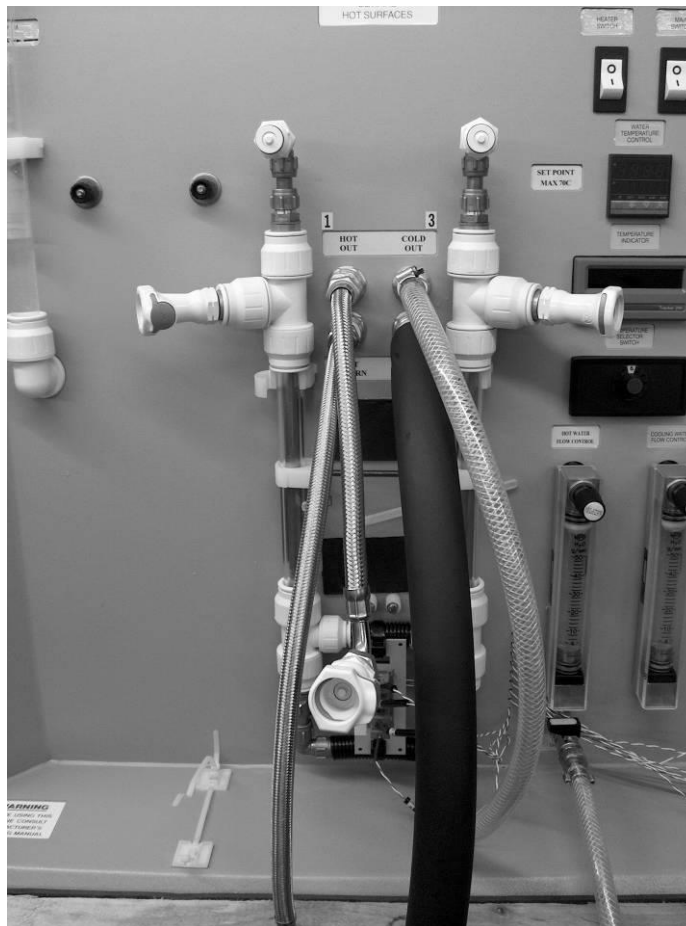
Fig. 6.1: Extended concentric heat exchanger connected to the service unit.
