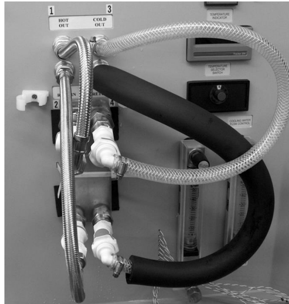
Fig. 7.1: Extended plate exchanger connected to the service unit.
